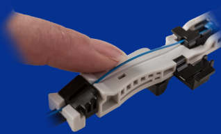
Check for fibre bend
